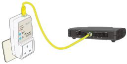
Connect the other PG902 to your computer, V-box or other network device using an Ethernet cable. This is the End Point (EP).
